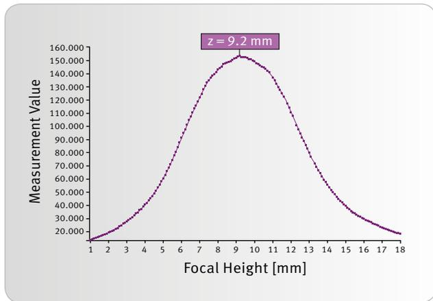
The automated focal height adjustment ensures the best signal-to-noise ratio in all detection modes and all plate formats.
