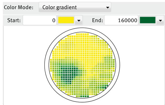
Well Scanning of GFP-expressing protoplasts. The well scan shows that the protoplasts (green colour) are not evenly distributed in the well.
