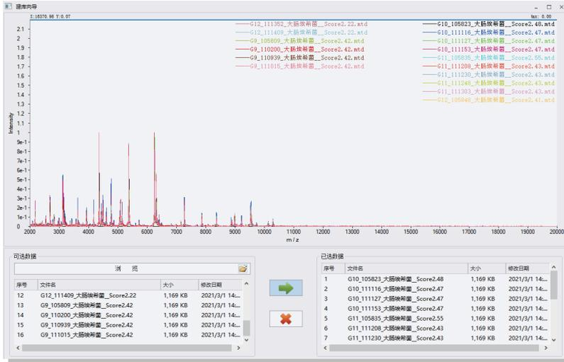
The system can intelligently identify and correct the  $\pm 10$  Da of the spectrum offset with synchronous searching during the process. And the detection result will be obtained within 0.1s.
